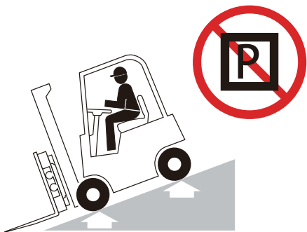
禁止坡上停车 No parking on ramp
